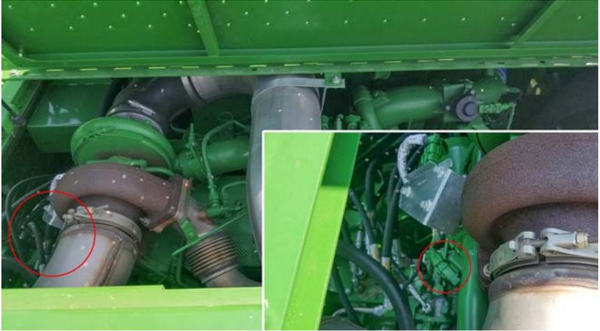
To locate the EGR pressure connector, lift the second access panel closest to the grain bin. The EGR pressure connector can be found under the cutout in the sheet metal panel as shown below.
